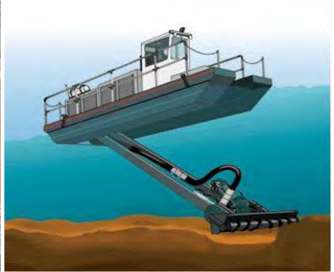
Picture of dredge in operation. Note the cutterhead at the front. Directly behind the cutterhead is the hydraulic submersible pump. Trailing behind the dredge is a floating pipeline used to transfer the biosolids to shore.
